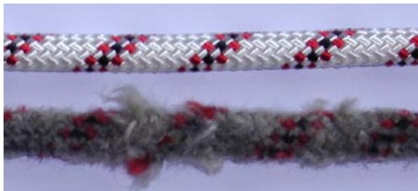
Fig. 2: Severe rope wear, wear with rope thickening
